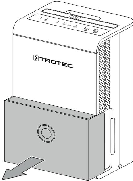
2. Empty the condensation tank over a drain or sink.
