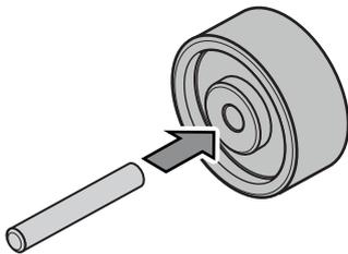
2. Tilt the device. Put a wheel into the mounts at the bottom of the device until it locks in place.
