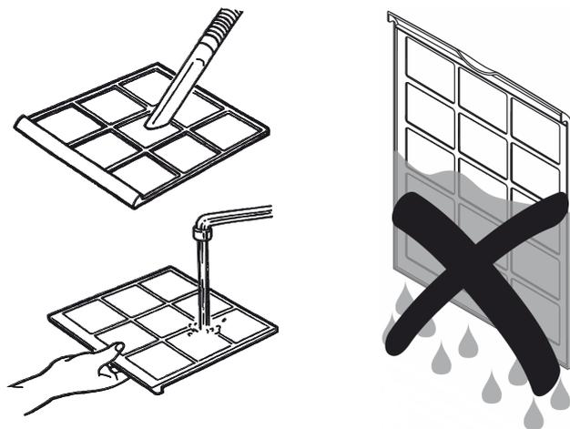
4. Allow the filters to dry completely. Do not put any wet filters into the device!
