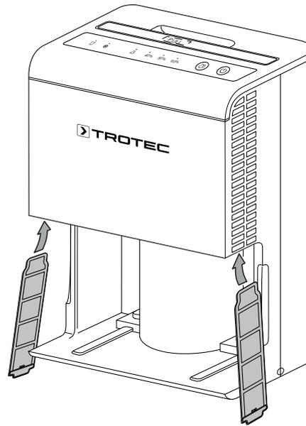
3. Clean the filters using a slightly damp, soft, lint-free cloth. If the filters are heavily contaminated, clean them with warm water mixed with a neutral cleaning agent.
