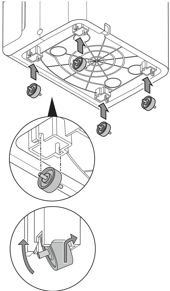
3. After mounting the wheels, place the device in an upright position.
