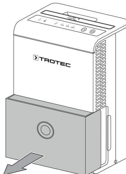
2. Remove the air filters from the device.
