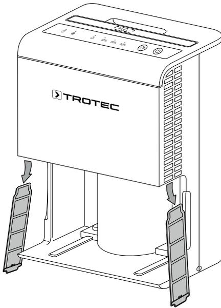
5. Reinsert the air filters into the device.
