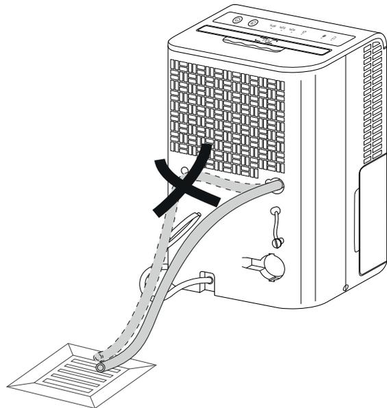
Remove the hose if you want to collect the condensate in the condensation tank again. Allow the hose to dry prior to storage. The hose can be connected in any operating mode for continuous operation.
