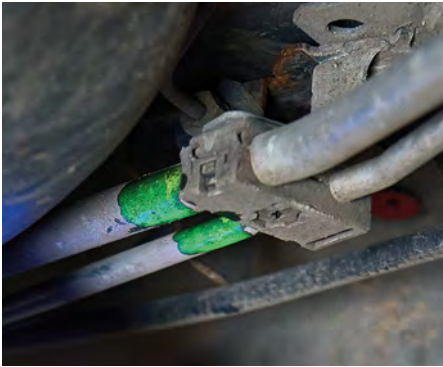
Leakage at the refrigerant line of a car's air conditioning system under UV light using a contrast medium.
