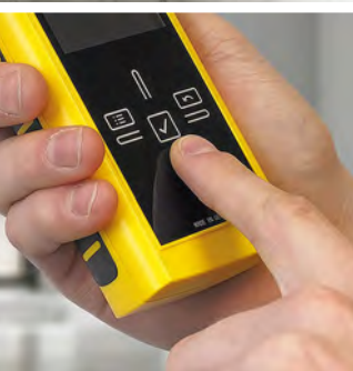
T210 and T260 come with a continuous surface made of highly scratch-resistant Blanview special glass and capacitive touchscreen control panel.
