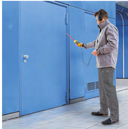
Combined with the ultrasonic transmitter SL800T, tightness tests of e.g. fire doors can be performed quickly and at low cost.
