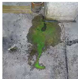
Uranin Green is already visible to the naked eye at the exit point, and fluorescence excitation via UV light can even produce quick tracer detection across large areas.
