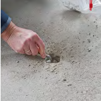
Step 1: As usual, a sample is taken of the entire cross-section of the screed and then placed in a bag.
