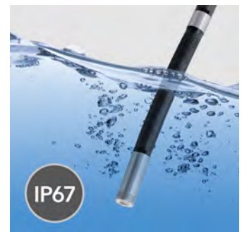
With a length of 1 m (ø 6 mm), the oil-resistant IP67 probe of the VSC106 offers maximum freedom of movement combined with high torsional strength due to its multi-layer construction of tungsten wire mesh and PU on a flexible steel spiral.
