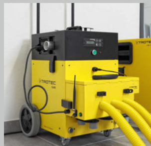
DRYING Insulation drying of wagon sandwich floors
